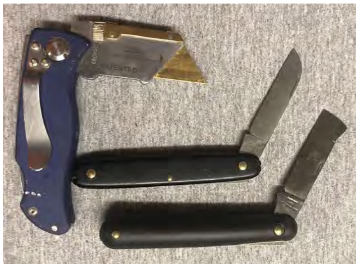
Figure 1. (From left) box cutter, grafting knife, and budding knife.
